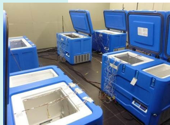
Fig. n°11 : Testing of refrigerators for vaccine storage in the framework of the WHO PQS programme.
